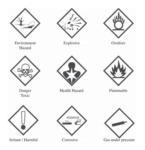
Hazard symbols shall have a black symbol on a white background with a red frame sufficiently wide to be clearly visible.
